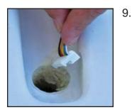
Feed the new connector through the installation hole. (Some controls have a protective cap over the connector. Put it back on now so the connector is not damaged as it travels through the channel).
