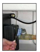
10. If the connector does not easily slide through the hole, feed a bent hanger up from the bottom...
