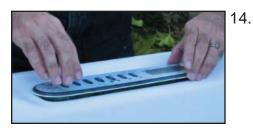
Press the new panel in place and re-connect the cable to the PC Board.
