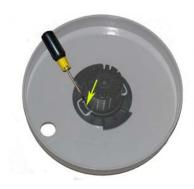
To clean the Inner Filter Screen, first remove the entire plastic Filter Screen as described above.
