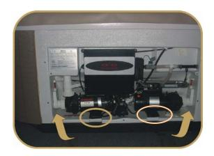
7. Remove the two shipping bolts located on the front of the pump mount (circled in illustration).
