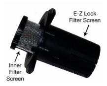
Then remove the Inner Filter Screen and clean both screens with water, using pressure from the **inside** of each screen.
