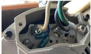
5. It is very unlikely that a new pump is defective upon installation. If your new pump is not working after installation, the most likely reason is improper wiring.
