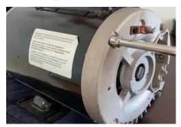
**5. Tighten the thru-bolts** (see picture from step 3) to secure the wet-end in its new orientation. Install the pump amp cord if not yet installed. Re-install the motor cover from step 2 if there was a cover to remove. **The pump is now ready to be installed!**
