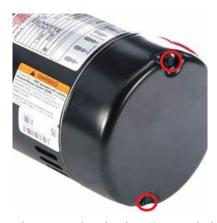
**4. Rotate the wet-end** in the direction needed for your plumbing. Pull out on the wet-end (away from motor) to allow for more space for rotation, and make sure to line up the bolt-holes with where the thru-bolts exit the motor and connect to the wet-end.
