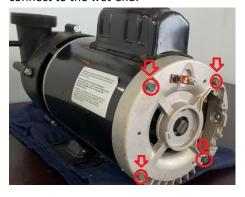
**3. Unscrew the thru-bolts** from the wet end, and pull them back until there is enough space for you to rotate the wet-end. You do not need to fully remove the thru-bolts, and it is not advised.
