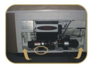
7. Remove the two shipping bolts located on the front of the pump mount (circle area). Then check to ensure that the gate valves (arrows) on the pump(s) are in the open position (handles fully extended).
