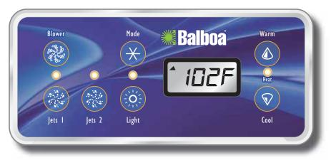
Serial Standard PN 53189-01 with Overlay PN 10430 • Connects to Main Board terminal J1
