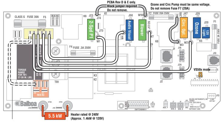
DIP A10 must be ON and jumper added for 120V systems. Remove for 240V Systems.
