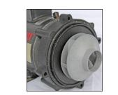
11. Wipe the ceramic disc seat with a clean rag, removing any old dirt or grime.
