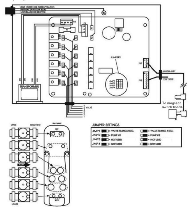
If the pc-board needs to be replaced, verify the jumper configuration is set for the correct pump.
