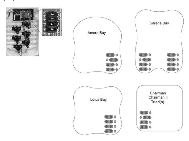
If a solenoid valve needs to be replaced, verify that the flow arrow is pointing to the correct direction. Normally they all point towards the equipment compartment.
