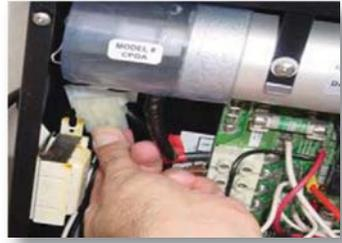
13. Turn on power at the GFCI again. Within a few minutes the Assembly light should come on, and you'll know it is operating. (A small percentage of units may not turn on. This probably means the transformer needs replacing too.)
