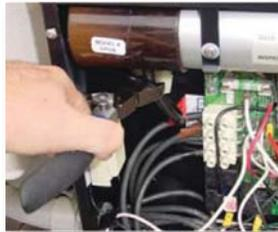
7. Remove both screws from black mounting strips. You will need to hold the tube assembly carefully from behind to insure it does not push against any other electrical components and cause breakage.
