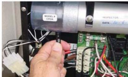
12. Move the white power connector off the left side of the P.C. Board and out of contact with any other electrical components. Failure to do this could cause shorting and damage to your spas' electrical system.
