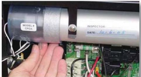
11. Over time, the vinyl hose becomes stiff and is difficult to re-attach. Carefully heat the last 1-2" of the black hose with a cigarette lighter until it begins to soften. It should then be easier to slide over the soapy barb. (Replacing the vinyl hose can be a bit trying, so just be patient and keep at it.)
