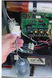
6. Cut vinyl hose from barbs on both sides of the old tube assembly. Use scissors or wire cutters to carefully snip as close to the barb as possible. Be careful not to cut any other wires in the equipment box. Sometimes the barb breaks off on its own. That works too!
