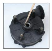
12. Using the screwdriver again, push the spring assembly out of the back plate.
