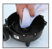
16. Wipe the white ceramic disc seat and face of the spring assembly with a clean rag, again to remove any fingerprints or other oils.
