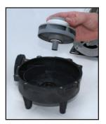
9. Separate the impeller from the back plate.
