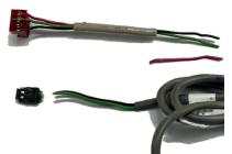
Note: If the special tool is not available, regular mechanical pliers can be used to crimp the connectors, by opening them to the "larger size".
