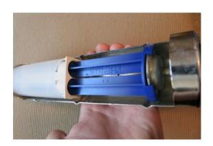
**Step 2**: Insert epoxy tube into barrel.
