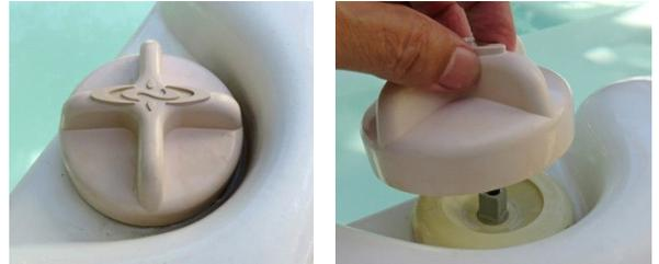
**Step 2:** Under the knob you will find a threaded cap. Unscrew and remove it. If the cap is difficult to turn, cover it with a towel and use a large pair of channel-lock pliers to get it started. Once the cap loosens, remove the towel and cap.
